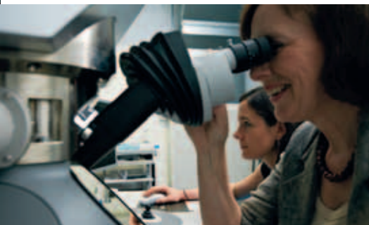
Atomic view: Professor Philip Withers and Dr Rob Bradley (left), in the Henry Moseley x-ray imaging facility, carrying out 3D x-ray tomography with a 50 nanometre NanoXCT microscope, which has the highest spatial resolution in the UK. Below: a PhD student in the Corrosion and Protection Centre conducting carbon dioxide testing in a cell within the controlled environment of a glove box. Bottom: Professor Grace Burke (foreground) and Dr Sarah Haigh operate the UK's only Titan G2 ChemiSTEM electron microscope.
