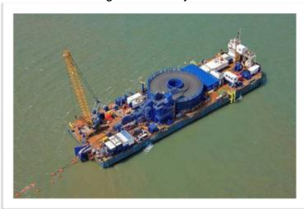
Figure 9: Cable on board an installation barge with dynamic turntable
