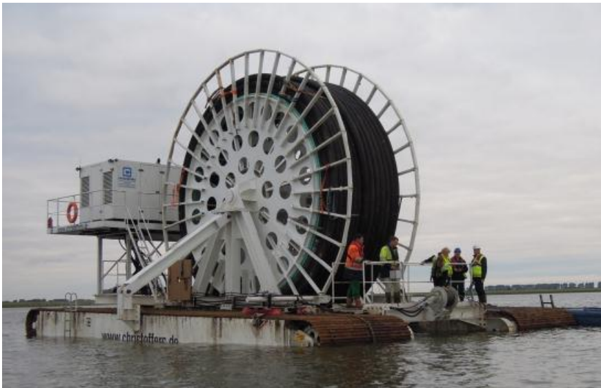
Figure 27: Modular transport vehicle with cable drum
