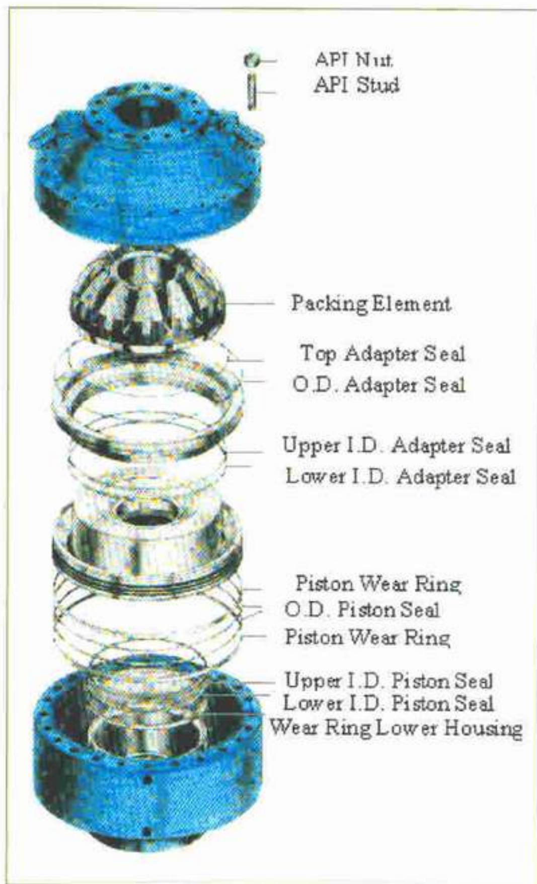
Figure5- Detail of packing unit
