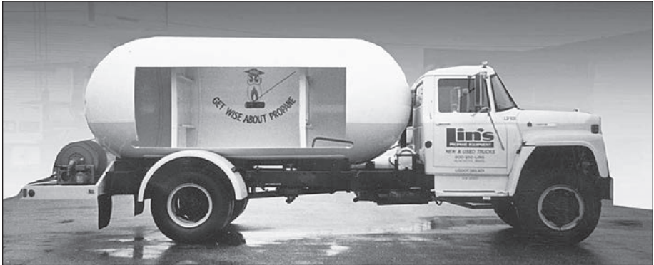
Fig. 7–2. Cutaway of a bobtail showing the baffles
