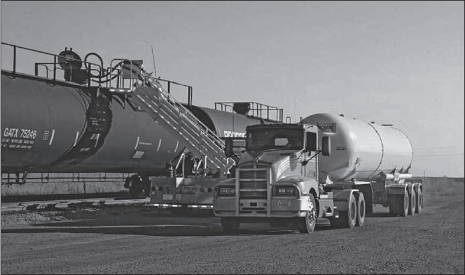
Fig. 7-3. A propane transport truck unloading from a pressurized tank car (courtesy of Westmor Industries)
