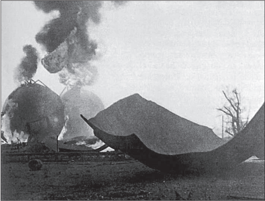
Fig. 10–6. Tank remnants from the San Juanico explosions (courtesy of Norwegian University of Science and Technology)
