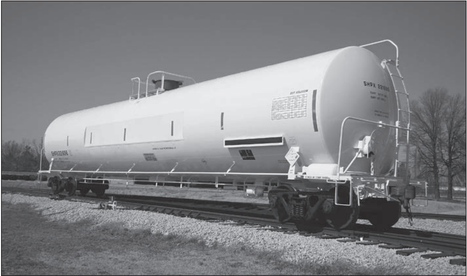
Fig. 7-4. Standard 32,500-gallon pressurized tank car (courtesy of American Railcar Industries)
