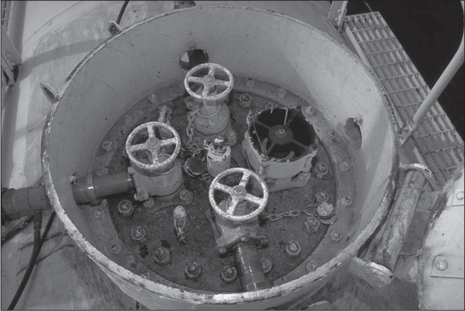
Fig. 7-5. Fittings in the dome of a propane tank car
