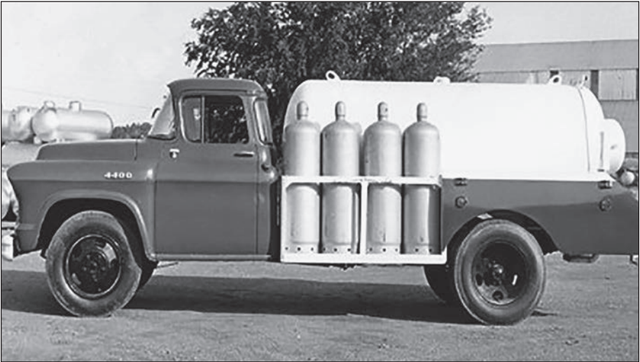
Fig. 2–5. A vintage propane bobtail. This truck from about 1950 delivered both bottled gas and bulk propane.
