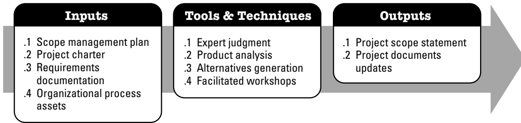
Figure 5-7. Define Scope: Inputs, Tools & Techniques, and Outputs
