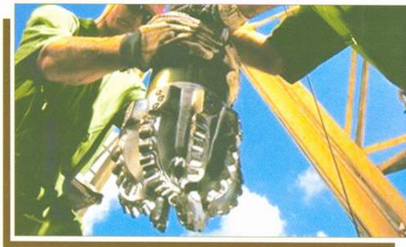
Fig 1. Drilling bit mounted on drilling string
