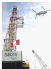
Heliportable Rig Ecuador/Peru
