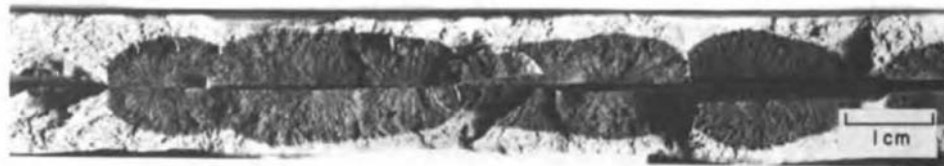
Fig. 2 Appearance of fracture surface of line pipe that failed by SCC. Actual size. See also Fig. 3 to 5.
