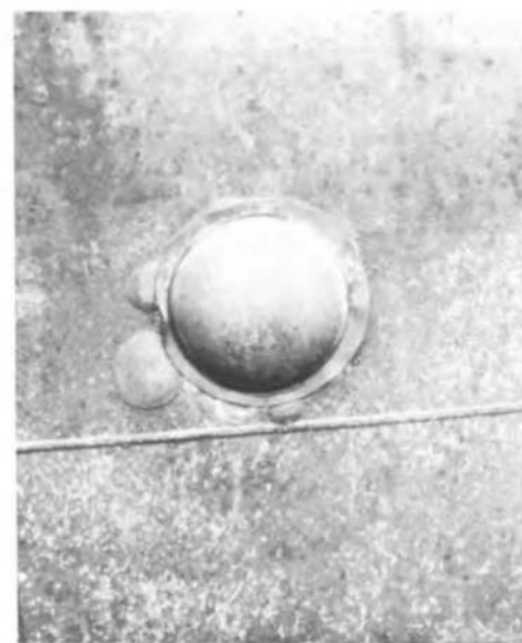
Fig. 12 Debonded organic coating near a high-silicon cast iron button anode
