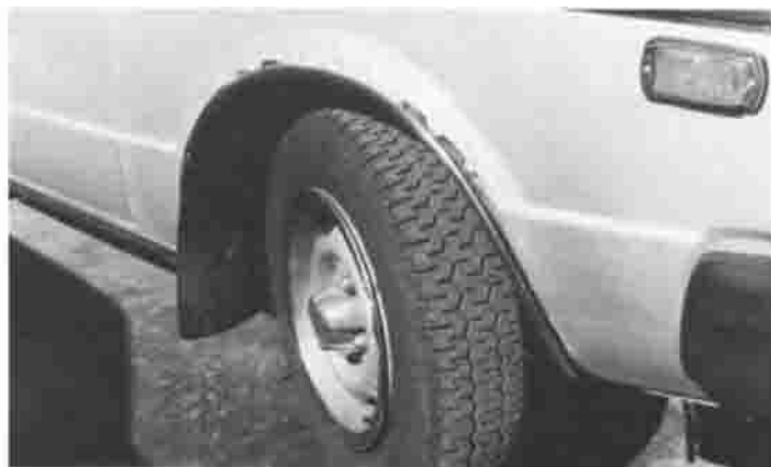
Fig. 12 Galvanic corrosion of painted steel auto body panel in contact with stainless steel wheel opening molding. Courtesy of R. Baboian, Texas Instruments, Inc.
