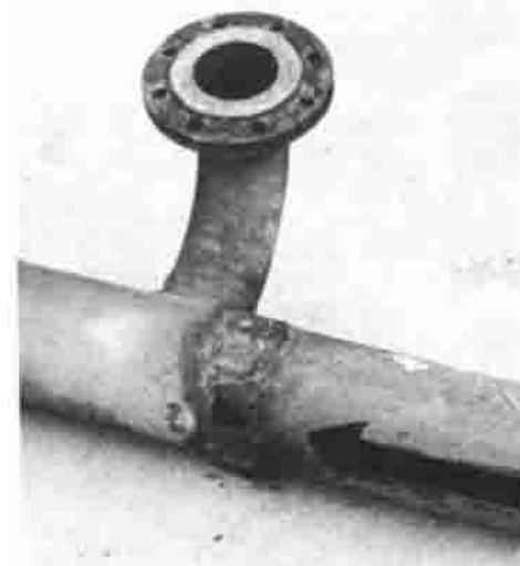
Fig. 9 Steel pipe corroded on the bottom side where a poorly sealed insulation joint allowed water to enter the insulation/pipe annulus. The moisture ran around the pipe and collected on the bottom.
