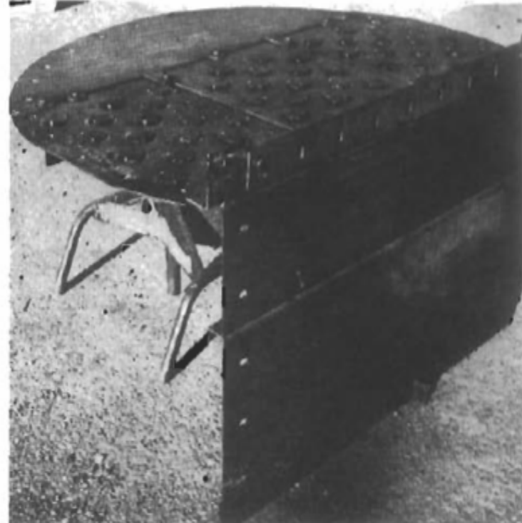
Figure 8-77. Type V-1 Ballast ® Tray. Used by permission, Glitsch, Inc.
