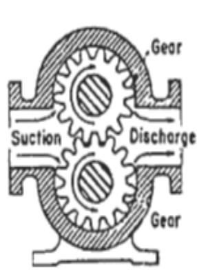
External Gear Pump
