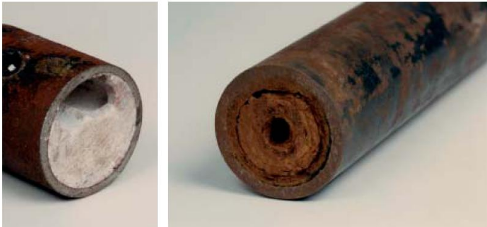
Boiler scale on water side
