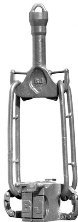
D-C Lift system employs (top to bottom) special adapter for drill pipe elevator, links, and collar type elevator for handling drill collars. Regular elevator latches around adapter when pulling drill collars from hole.
