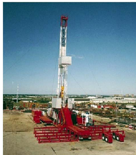
- Land Rig: Fast Moving Trailer Mounted
