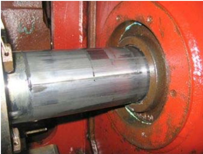
Figure 7 - Typical wiper seal.
