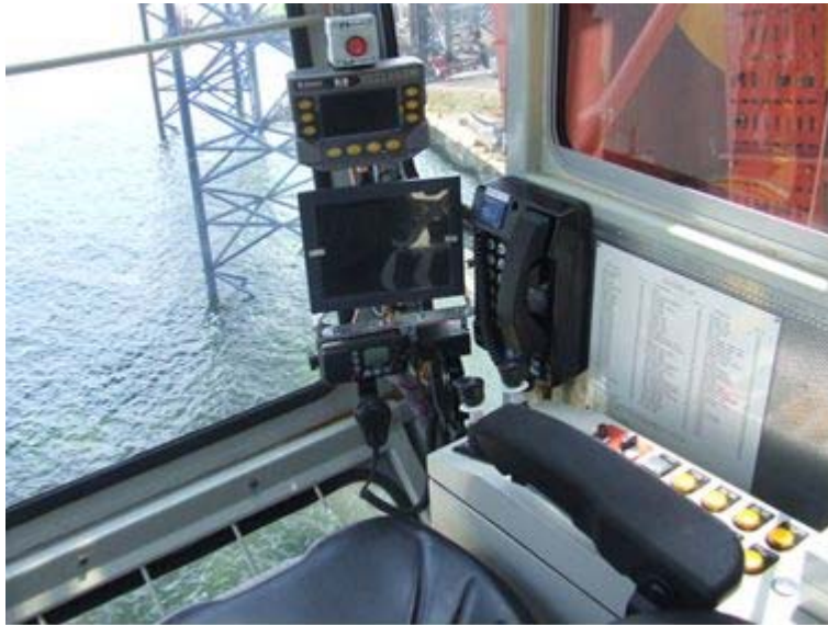
Figure 24 - Typical crane cabin.
