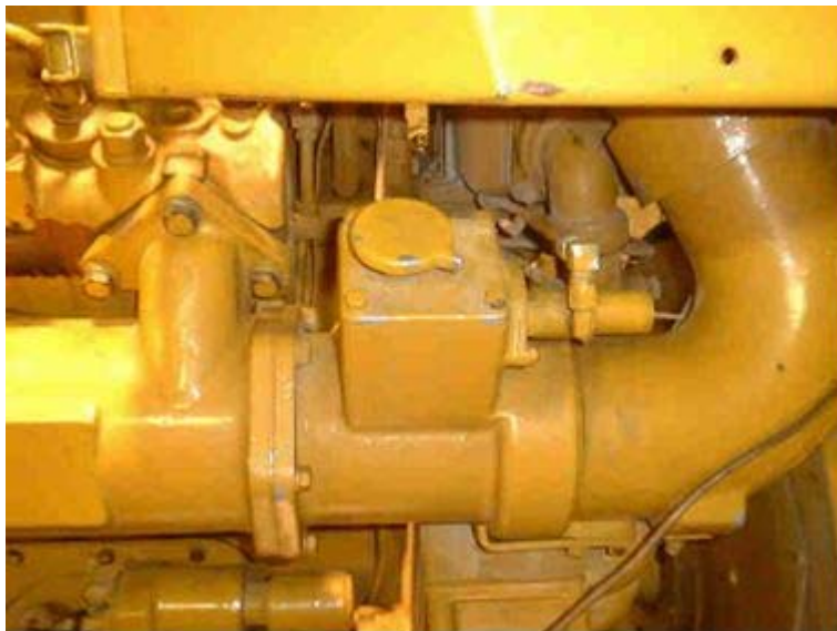
Figure 5 - Example of a rig saver valve.
