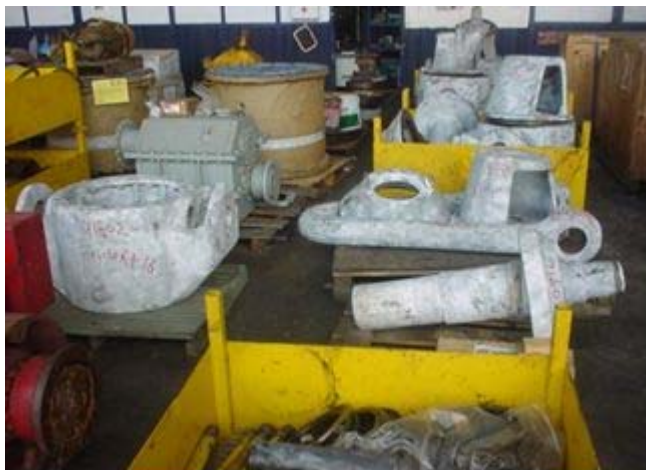
Figure 18 - Swivel stripped for API Category IV inspection.
