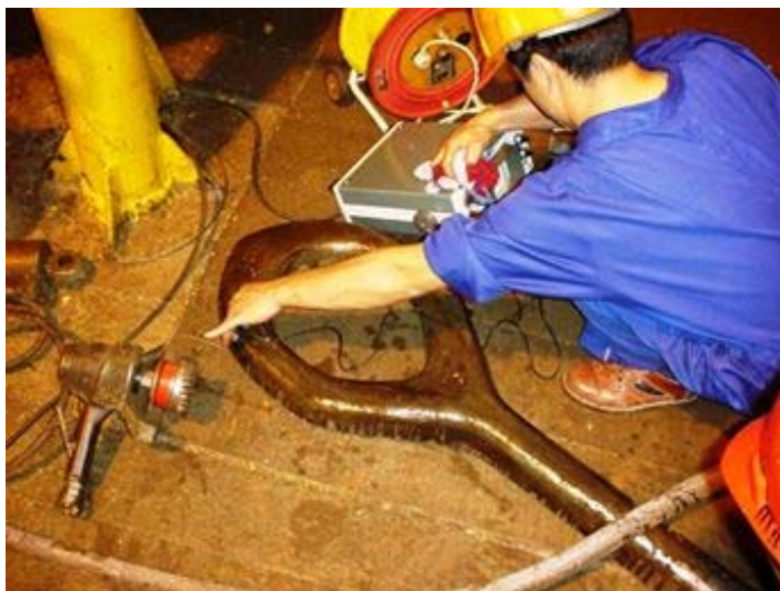
Figure 49 - Measuring the elevator bails/links.
