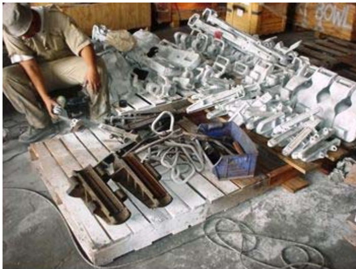
Figure 48 - Lifting gear under inspection.
