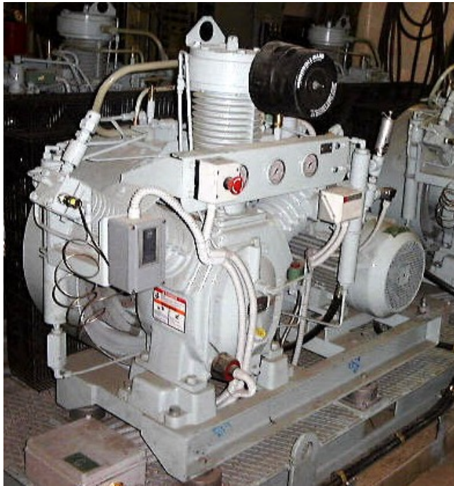
Figure 12 - Reciprocating air compressor.
