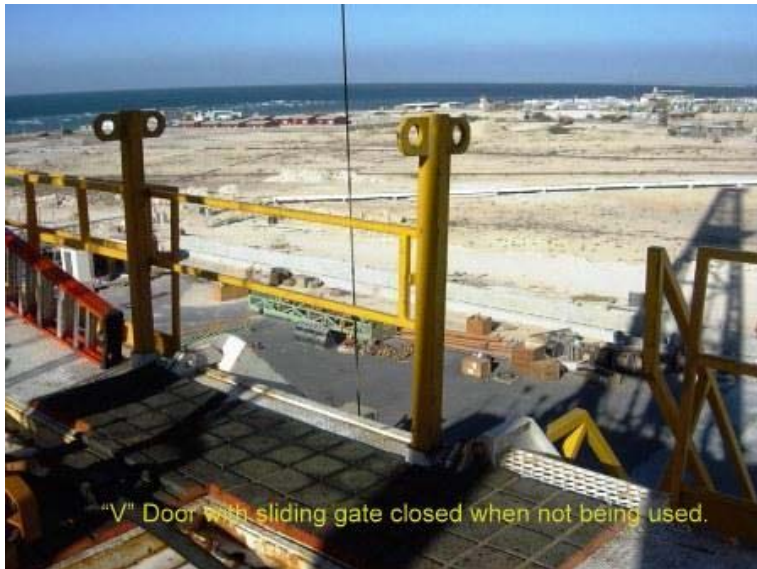
Figure 5 - V-door with sliding gate.
