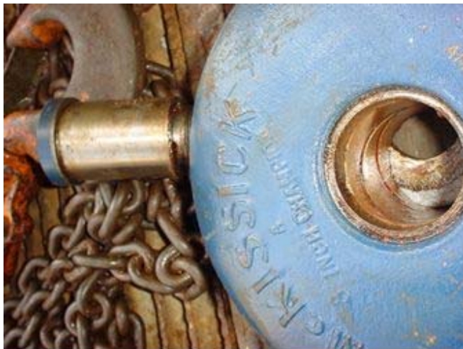
Figure 42 - Sheave undergoing inspection.
