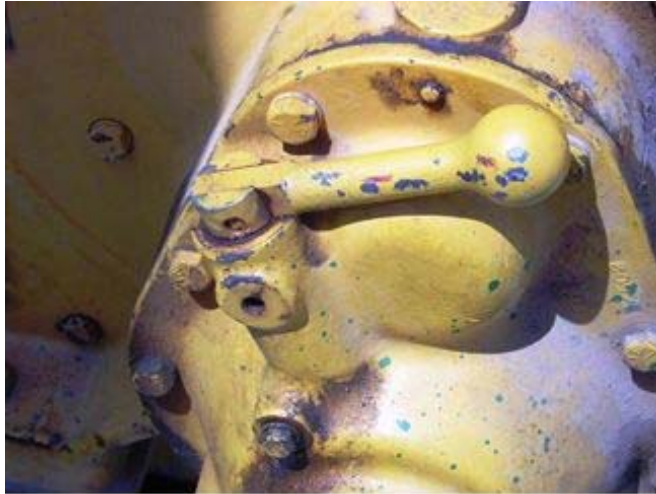
Figure 41 - Free-fall handle needs to be locked.
