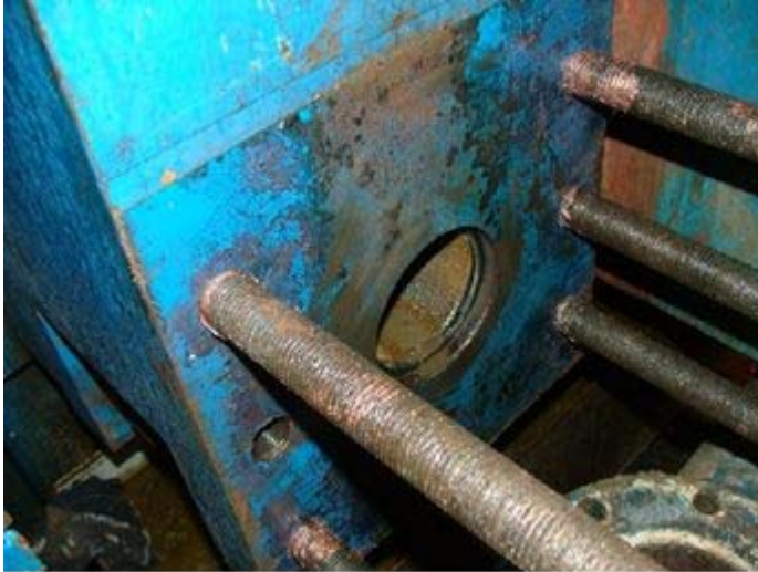
Figure 6 - Fluid-end studs should be inspected regularly.
