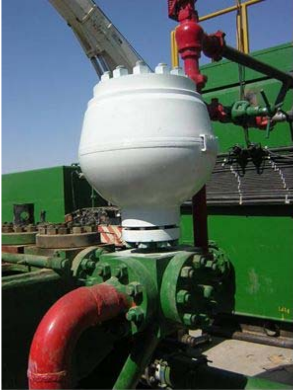
Figure 4 - Mud cross with strainer, pulsation dampener and relief valve.
