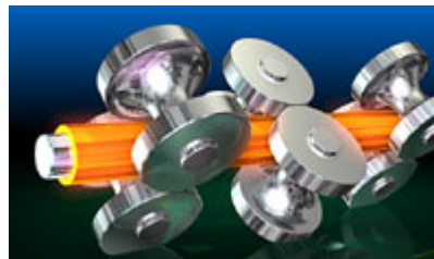
Tube rolling in continuous mandrel mill
