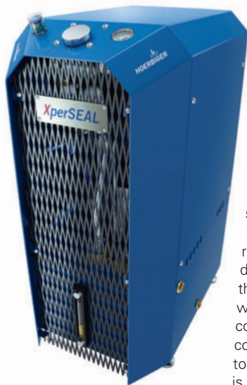
Figure 4: The central oil supply unit incorporates an oil pump, oil cooler, and functions for control, monitoring and safety
