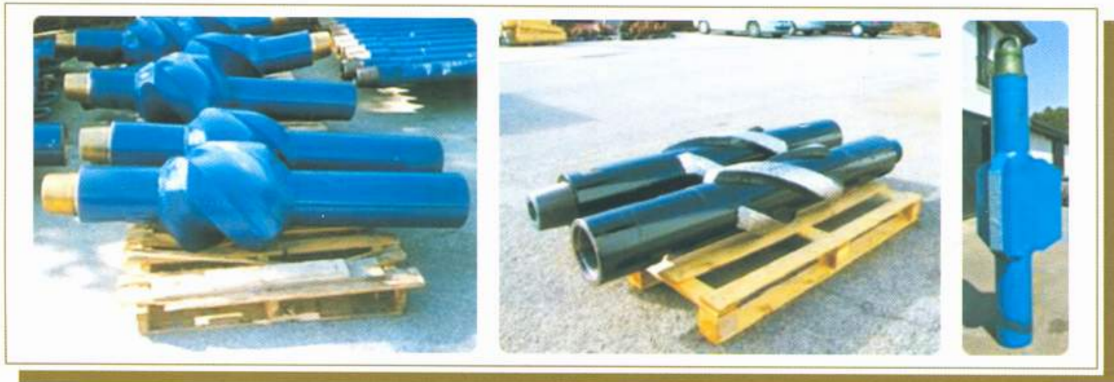
Fig.7. Spiral welded blades and straight welded blades Stabilizers
