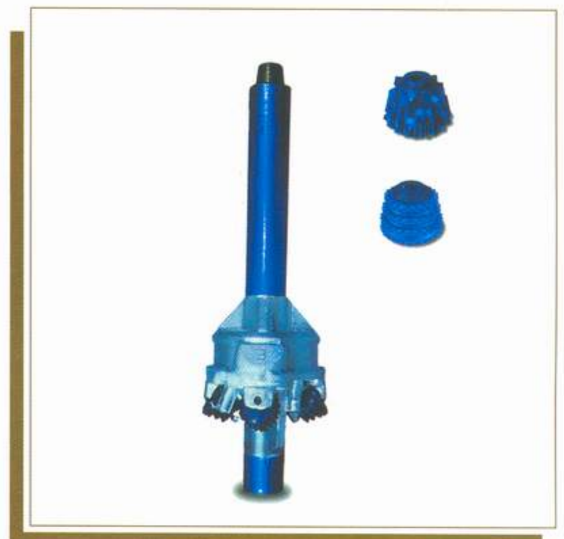
Fig.10. Five-cone hole opener
