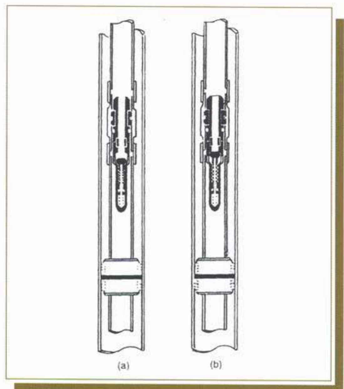
Fig.53. Pressure operated safety valves
