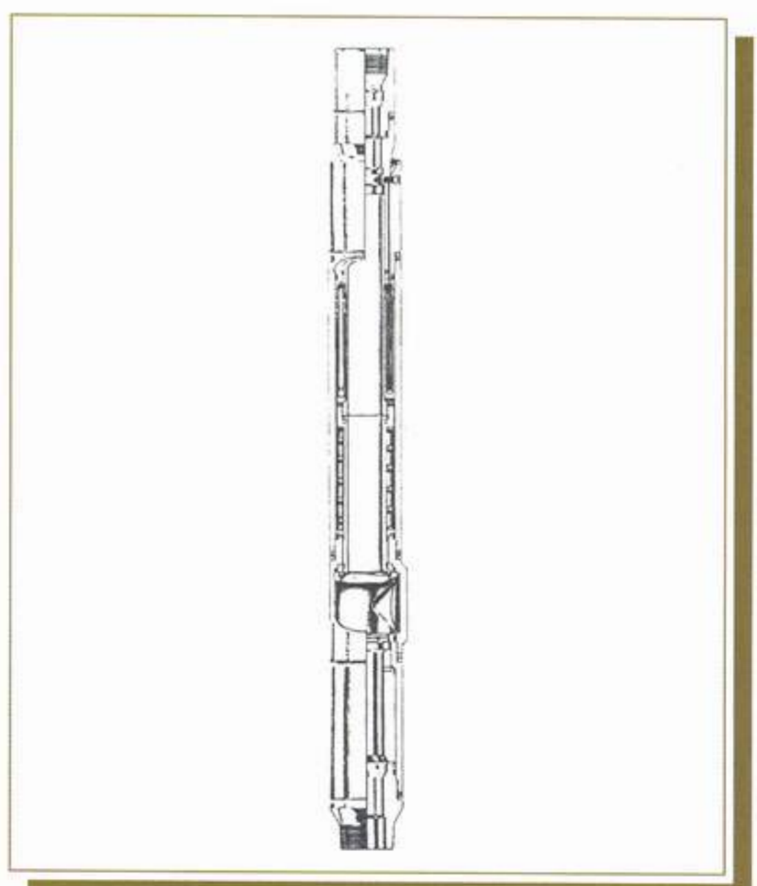
Fig.55. Tubing Retrievable safety valves
