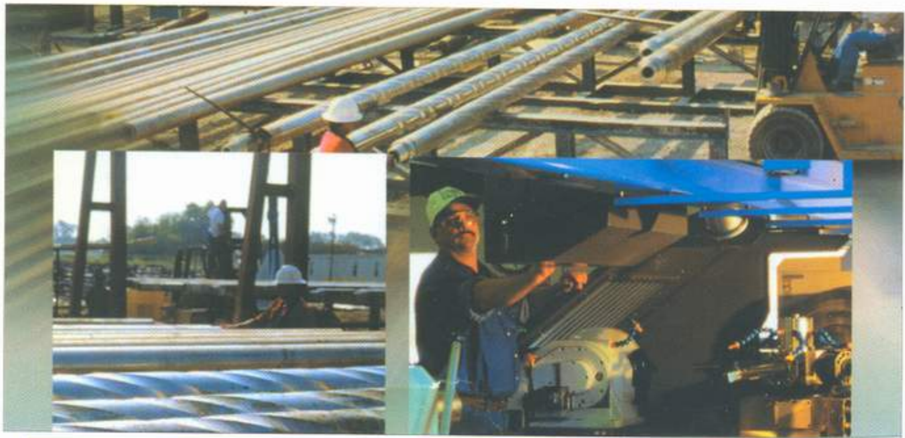
Fig.3. Spiral grooved drill collars
