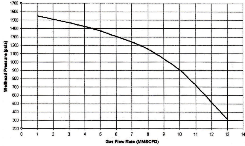
Wellhead Performance Curve for Well A
