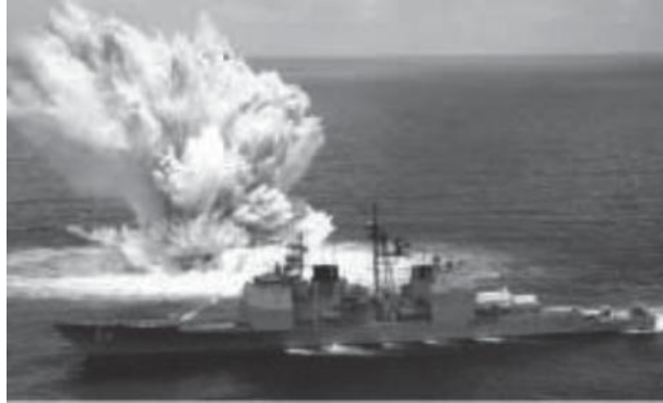
FIGURE 5.5 Naval shipbuilding materials require strength, weldability, fire resistance, and fracture toughness under sudden explosive shock loads. (From E.J. Czyryca et al., 2003, Meeting the challenge of higher and lighter warships, Advanced Materials and Processes Technology Information Analysis Center [AMPTIAC] Quarterly , Vol. 7, # 3, pp. 63–70.)
