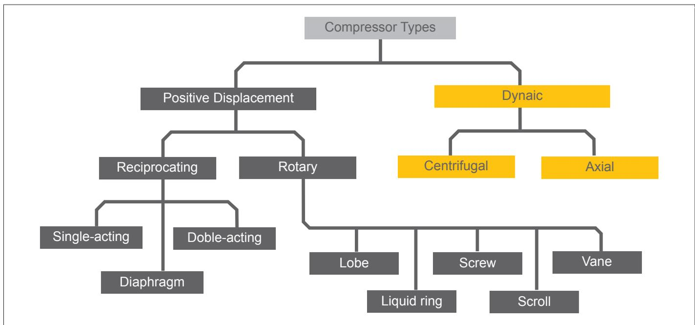
Figure 7.4 – Overview of compressor types.
