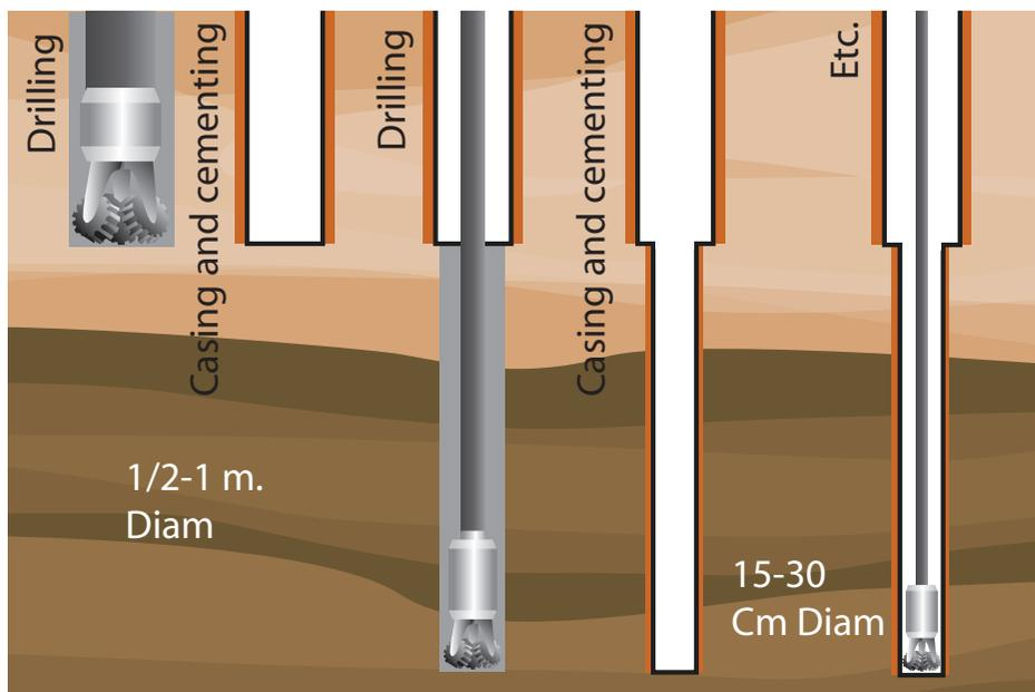
Figure 4.1 – Drilling of a well.
