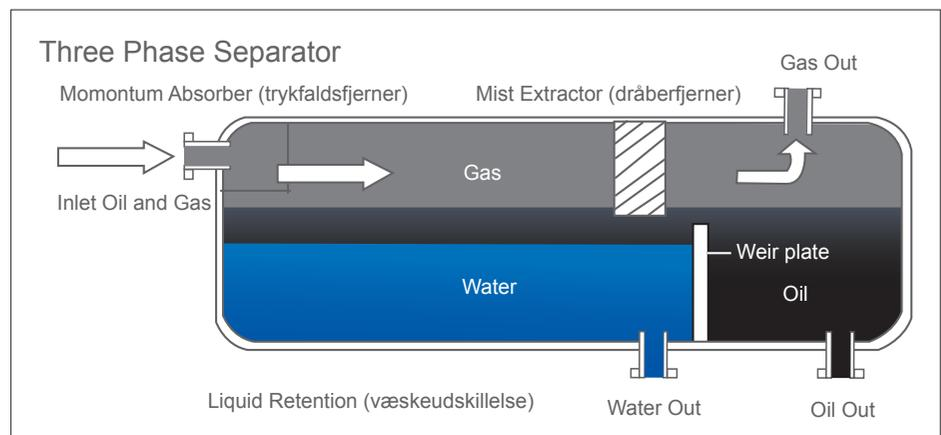
Figure 7.2 – Three-Phase Separator..
