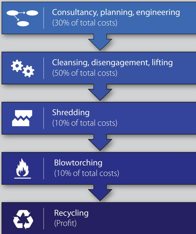
Figure 11.6 – Break down of decommissioning costs. Courtesy: Offshoreenergy.dk
