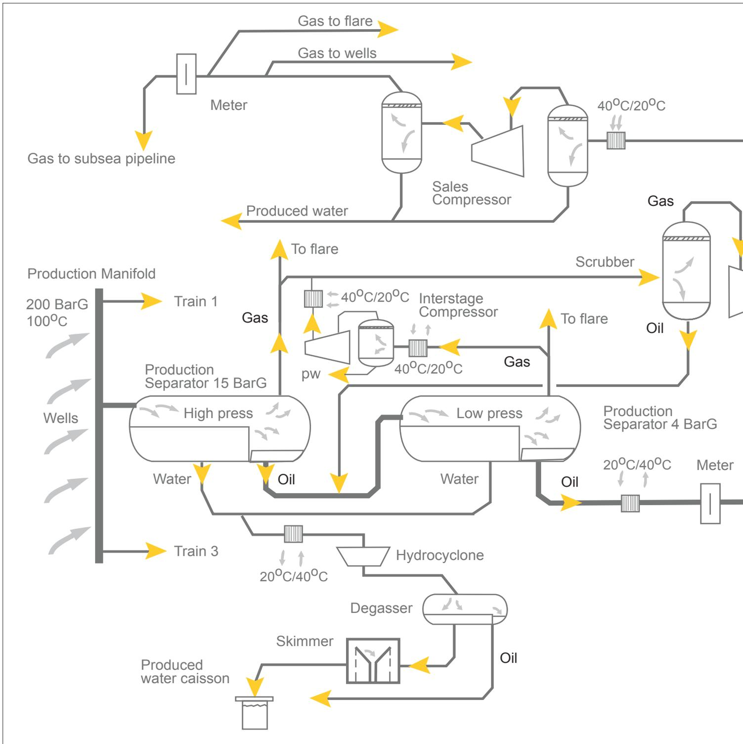
Figure 7.1 – Process Diagram illustrating the oil's way from the wellbore to pipeline.
