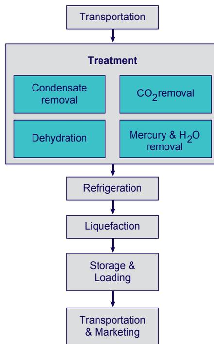
Figure 13.2 - A typical LNG process
