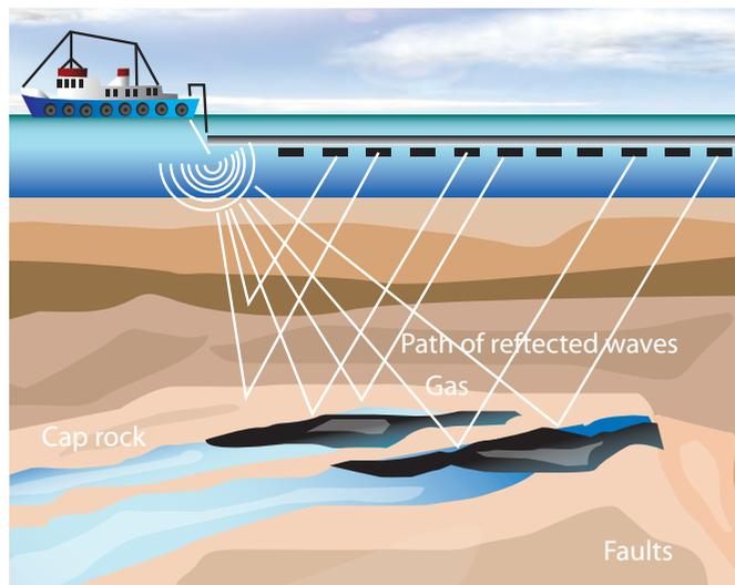
Figure 3.3 – Illustration of seismic survey.
