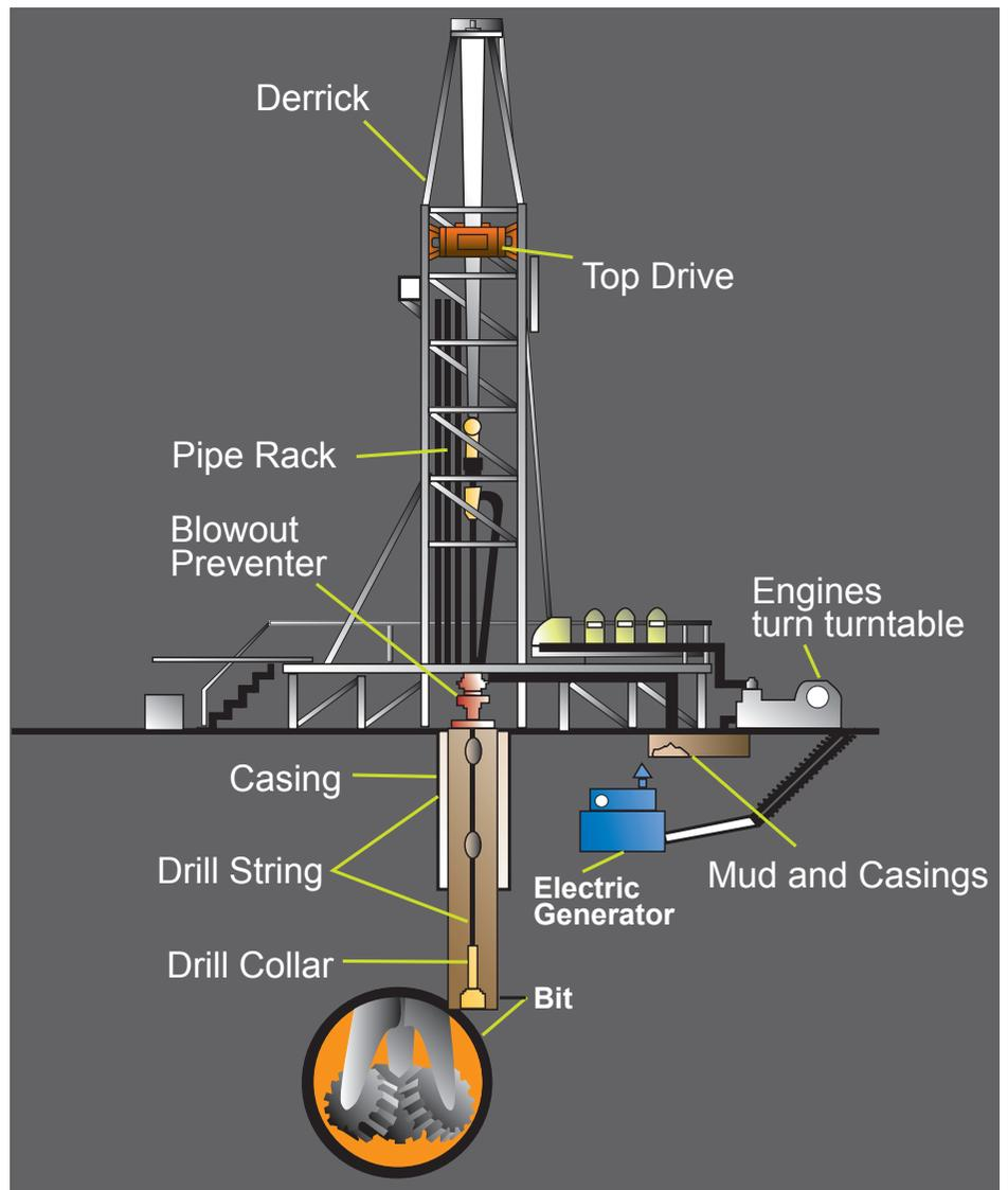
Figure 4.2- Drilling set-up.
