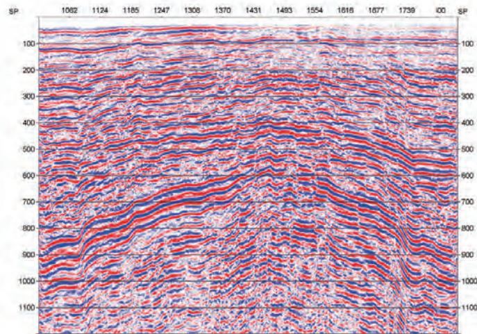
Figure 3.4 – Sample 2-D marine seismic lines. The lines are merged from individual shots (along the X-axis), and the Y-axis displays the time in thousands of a second it takes the seismic wave to travel from the surface to a reflector and back again.
