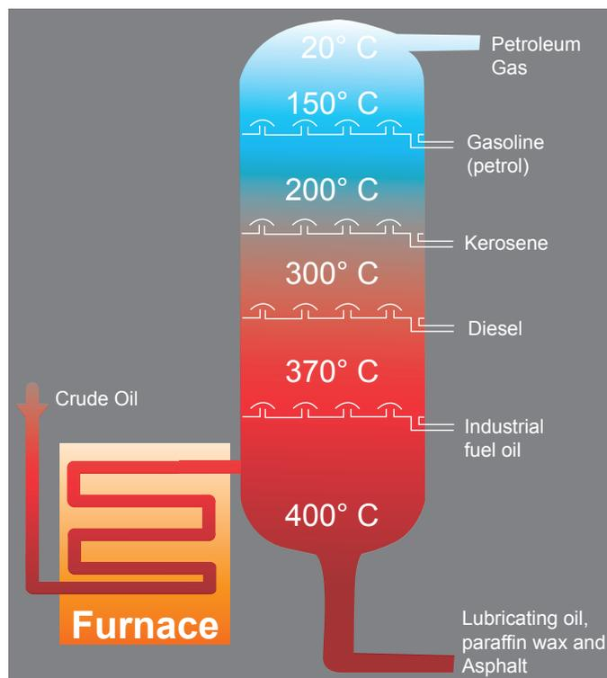
Figure 13.1 - Fractional distillation of crude oil.
