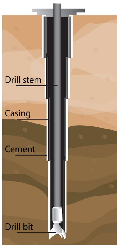
Figure 4.5 – Drilling of a well.
