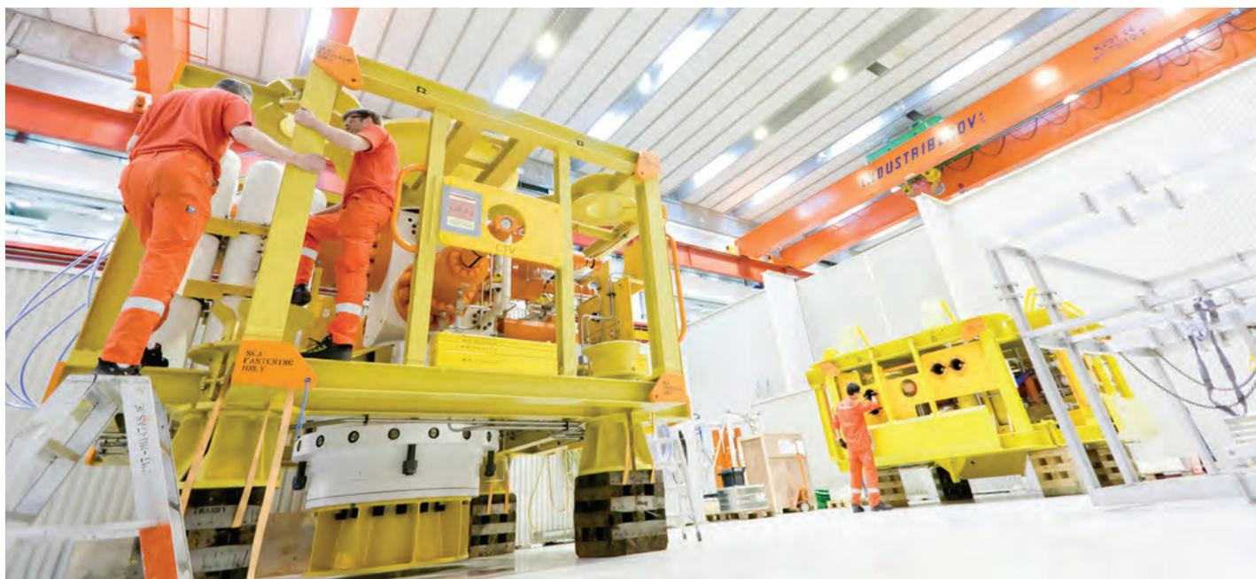
Figure 6.1 – A subsea Christmas Tree prepared for shipping. Courtesy: AkerSolutions
