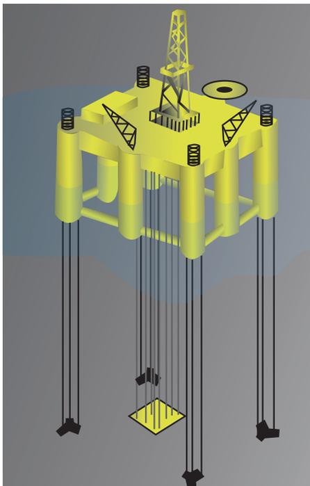
Figure 5.6 – Tension leg platform.
