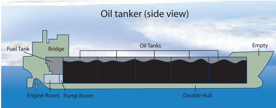
Figure 12.4 – Side view of an oil tanker.
