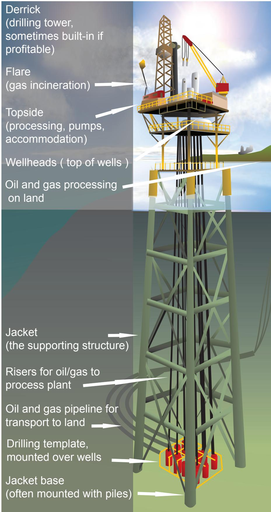
Figure 5.1 – Offshore Platform.
