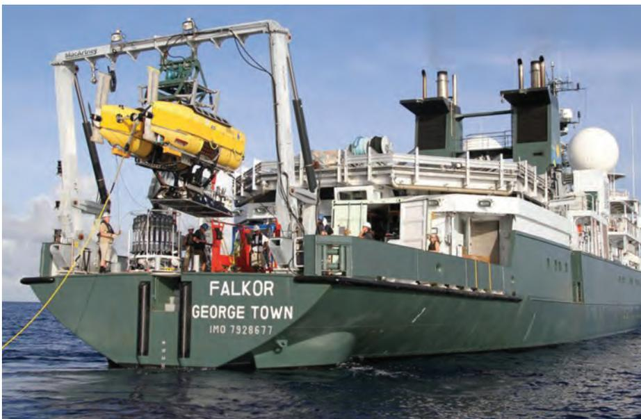
Figure 6.2 – Preparing for subsea operation with a ROV – Remotely Operated underwater Vehicle. Courtesy: MacArtney.
