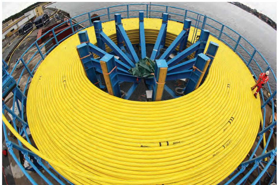
Figure 6.4 - Umbilicals prepared for installation. Courtesy: AkerSolutions.
