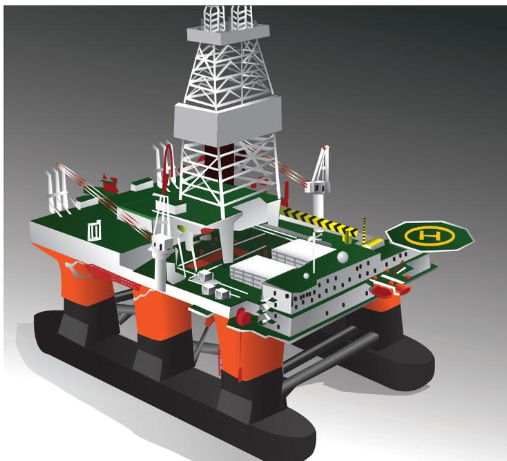
Figure 5.5 – Semi-submersible Platform.
