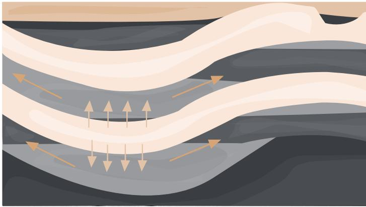
Figure 2.5 – Migration. Movement of hydrocarbons in the porous rock
