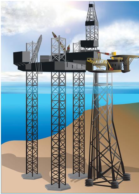
Figure 5.8 - Jack-up Platform standing next to a stationary platform.
