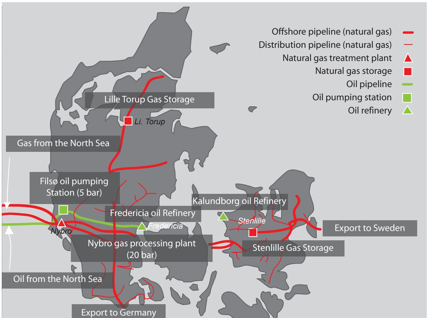
Figure 12.6– Onshore oil and gas transmission system in Denmark.
