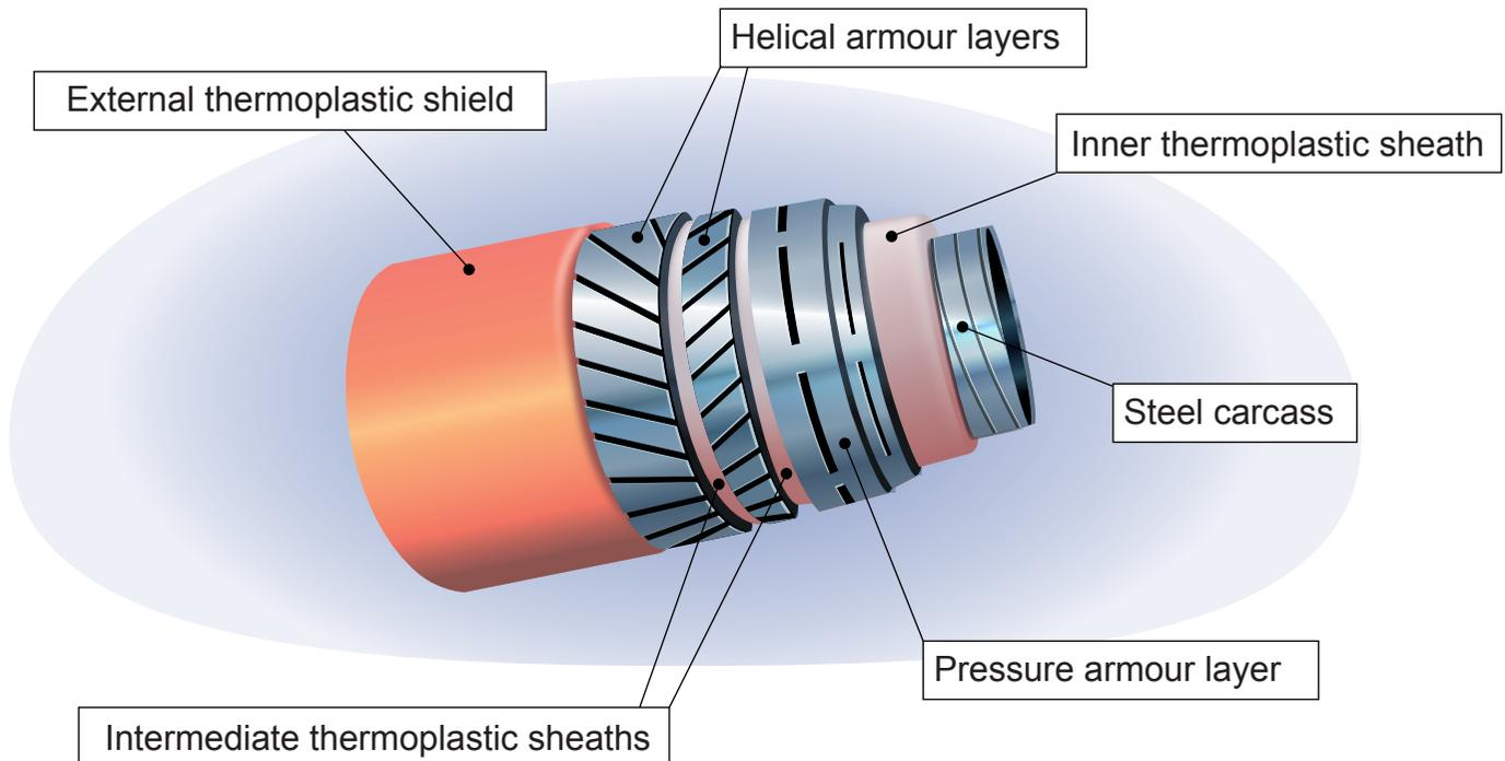
Figure 8.2 – Typical flexible composition.
