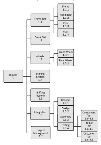
Figure D-4. WBS Horizontal Tree Structure View
