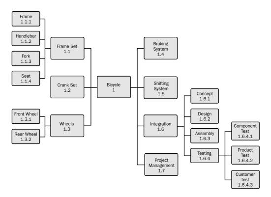
Figure D-6. WBS Centralized Tree Structure View 2
