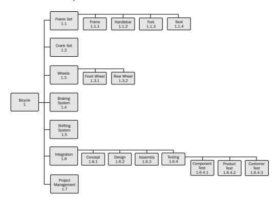
Figure D-2. WBS Tree Structure View 2
