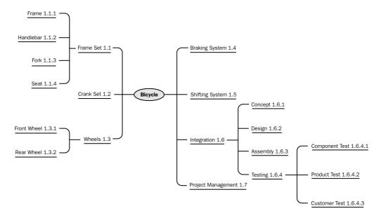
Figure D-5. WBS Centralized Tree Structure View 1
