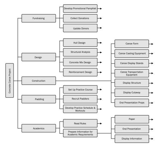
Figure P-1. Horizontal Tree Structure Format WBS Example
