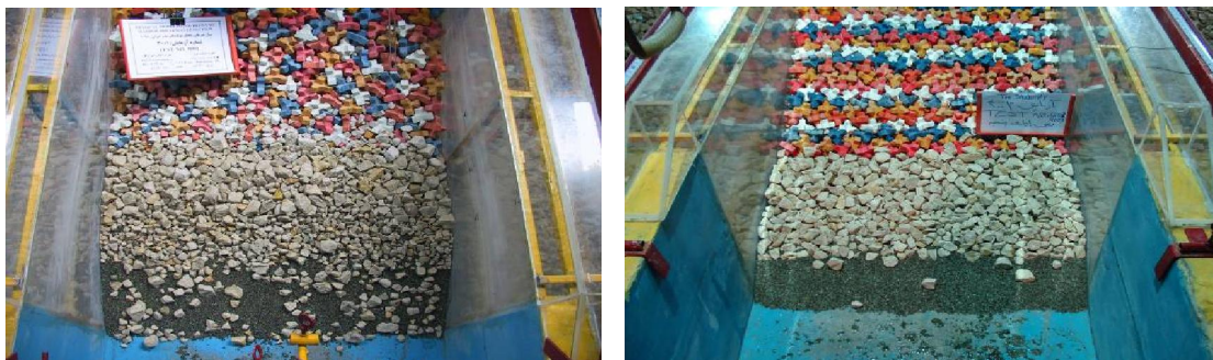
Fig. 11) Comparison of the Reshaped toe Berms (Left, Test No. 3001, section B8-B8-A and Right, Test No. 4003, section B8-B8-B)
