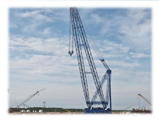
"The market continues to demand higher capacity machines to accommodate accelerated construction methods," says Ashton. Features distinguishing the AFRD are "high speed performance machinery for slewing, hoisting and booming, exceptional and unmatched capacity at radius, automatic self levelling, state-of-the-art safety features, Modular components for ease of assembly and economical transportation," Ashton explains.
